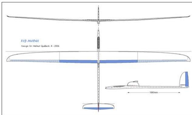
The left graphic shows the 3 side-draft for a new **F3J**-model designed by the author. Flight-mechanical characteristics of the model as given below have been determined by means of the “**FMFM**”-program (*Flight-Mechanics for Flight-Models*) which is described in more detail on the homepage [www.hq-modellflug.de](http://www.hq-modellflug.de).
