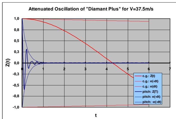
As we see, the fast pitching-oscillations very soon come to rest, whilst the c.g.-oscillations take a long time and can easily be balanced out by RC-control.
