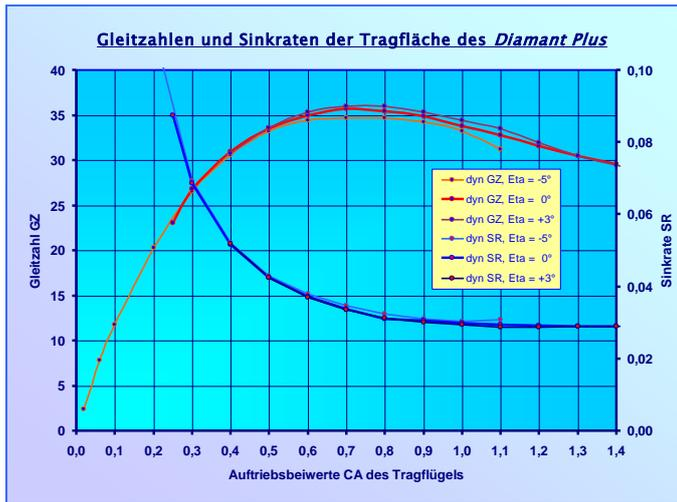
allow to deflect the wing-sections as desired for any flight state from very slow to very high speed. By means of the left graphic showing gliding numbers and sinkrates for the lifting wing of the “*Diamant Plus*” including induced drag, the aerodynamic working point was chosen to be at  $c_l = 1.2$  for good thermal soaring.
