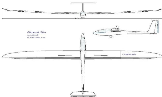
From the original "Diamant" the fuselage was used for practical reasons und thus the momentum-arm of the model was predetermined. In our home-page [www.hq-modellflug.de](http://www.hq-modellflug.de) one can find all details about the design aspects for the new development.
