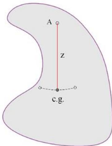
A simple practical method to determine the mass-moment of inertia of any given body is the following; If a body like that in the left graphic is equipped with an axis through A it can be stimulated to swing around this axis and the time  $T$  for one full period of oscillations is given by
