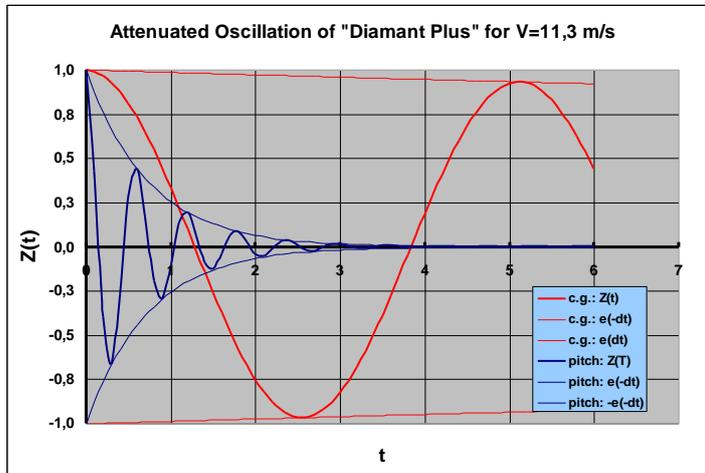
Here we have the typical behaviour of a model with a rather high mass-moment of inertia. While for the previous lower-weight F3J-model the fast pitching-oscillations already came to rest after about one cycle, here it takes about 4 - 5 cycles.
