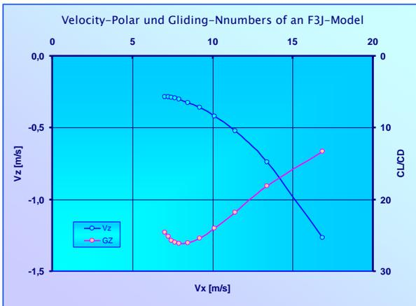
Finally, the left graphic provides the quasi-stationary theoretical performance parameters of the complete F3J-model for its expected operational flight range under inclusion of all sorts of drag related to the model.
